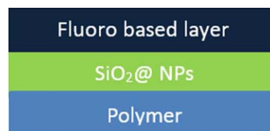
Scheme 1. Schematic presentation of proposed three layer composite superhydrophobic coating. [Color figure can be viewed in the online issue, which is available at wileyonlinelibrary.com .]
